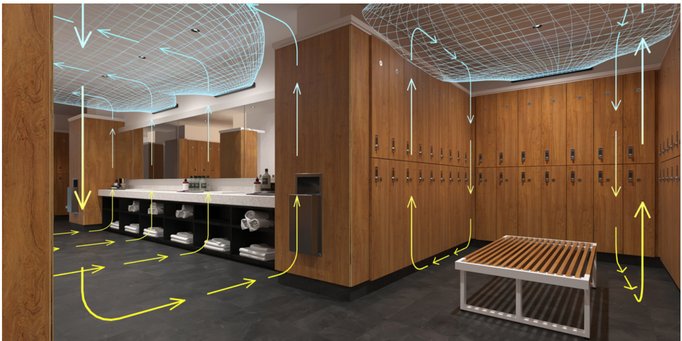
Figure 2: An upper air UVGI application illustrating UV distribution and air mixing.
