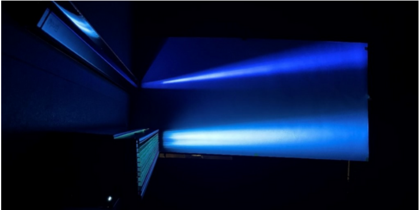
Figure 6: Beams emitted from a Purifii AER W (top) and a traditional low-pressure mercury upper air fixture (bottom).
